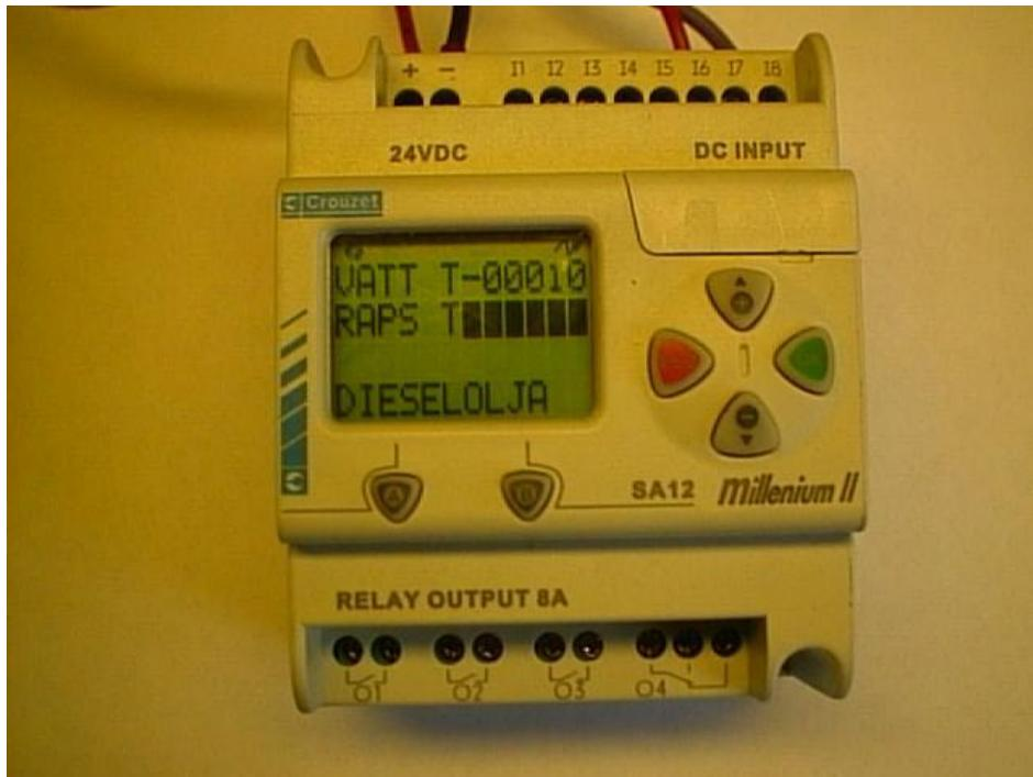
It is easy to mount PLC. You only mount cables from sensors and parts
